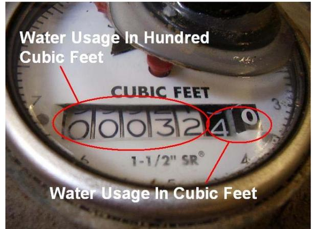
The leak indicator on the face of the meter is used to show small amounts of water that are flowing through the meter. If you focus on one corner of the black triangle, it will turn when even the slightest amount of water passes through the meter. If everything inside and outside the house is turned off, (like washing machines, faucets, toilets) and the leak indicator is turning, there could be a leak somewhere inside or outside the house.
